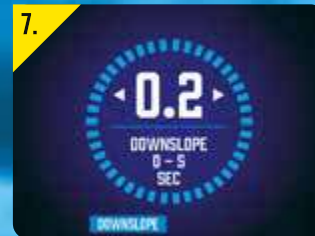
7. DOWNSLOPE Adjustment Screen (TIG Only)
